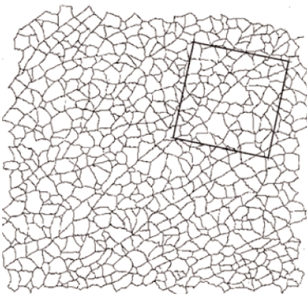
Figure C.3 — Mark and count the central particles and add these to the perimeter count to obtain the particle count for the specimen
